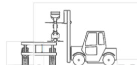
7.1.2 Using a forklift truck to load/offload
