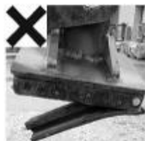
Damage causing the Rubber Strip to come away from the Brackets.
